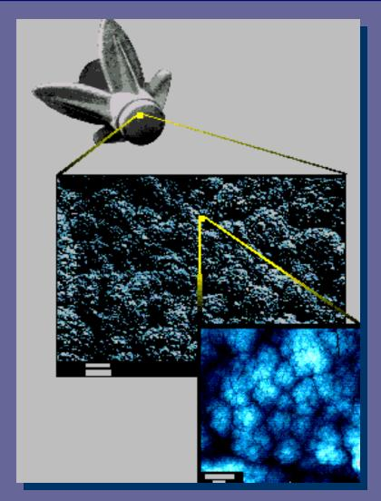
The "Cauliflower" structure of a fractal coated electrode tip (self repeating structure)
